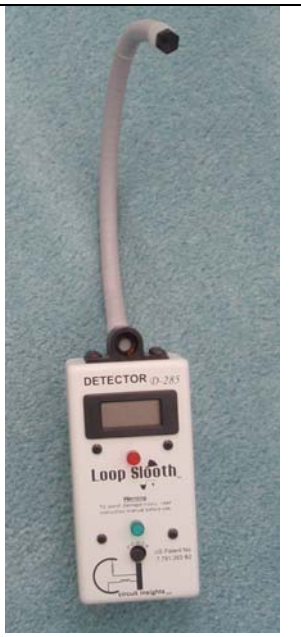
Figure 5. D-285 Detector with Rogowski coil untucked.
